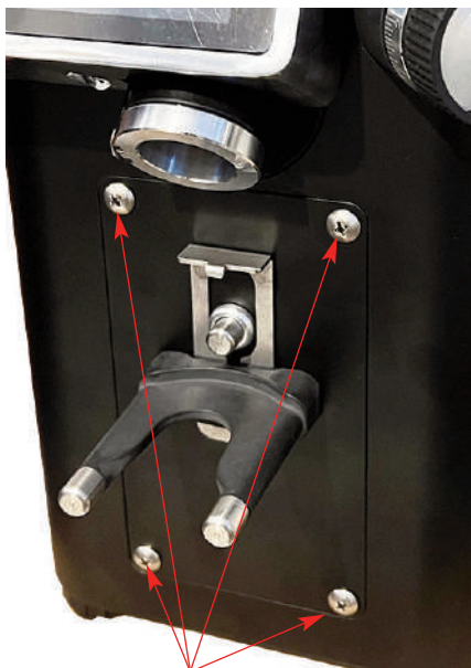
Unscrew the 4 screws of the module
